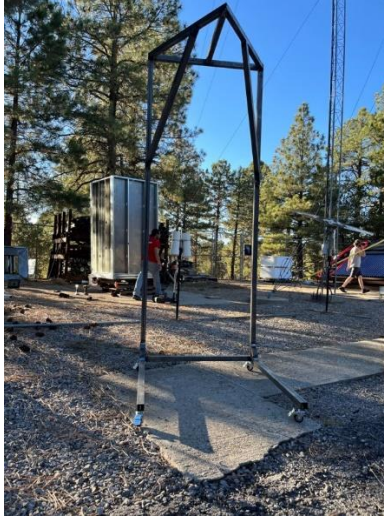
Figure 32: Rack System of Powder Coating Oven
