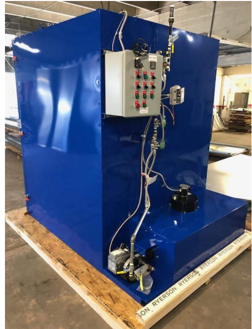
Figure 4: EPTEX Gas Oven PID and Heater
