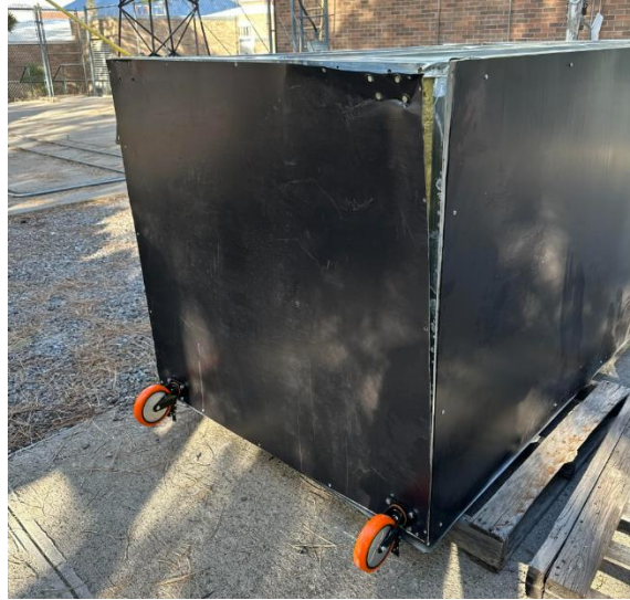
Figure 35: Results of Buckling Powder Coating Oven
