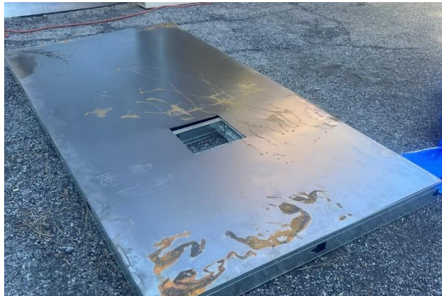
Figure 36: Oven Door with Hole Placement for Window
